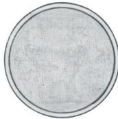
Erosion still permissible, plate can be polished
