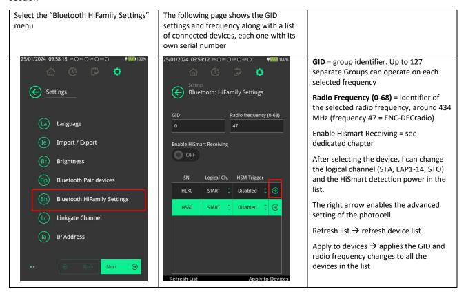
When the photocell is selected in the list you hear a double beep and the status LED blinks to signal which photocell you are working on.
