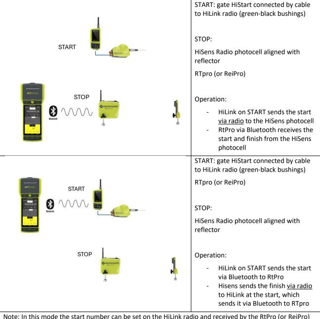
Note: In this mode the start number can be set on the HiLink radio and received by the RtPro (or ReiPro) stopwatch, while the Hisens photocell only transmits the pass (unless using HiSmart)
