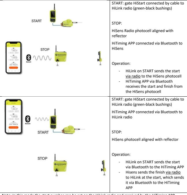
Note: In this mode the start number can be set on the HiLink radio and received by the HiTiming APP, while the Hisens photocell only transmits the pass (unless using HiSmart)
